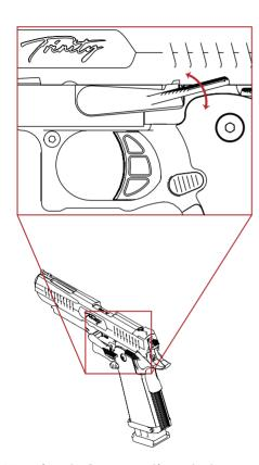
BY moving the lever to adjust the hop-up. Clockwise to increase the hop-up. Counterclockwise to decrease the hop-up.
